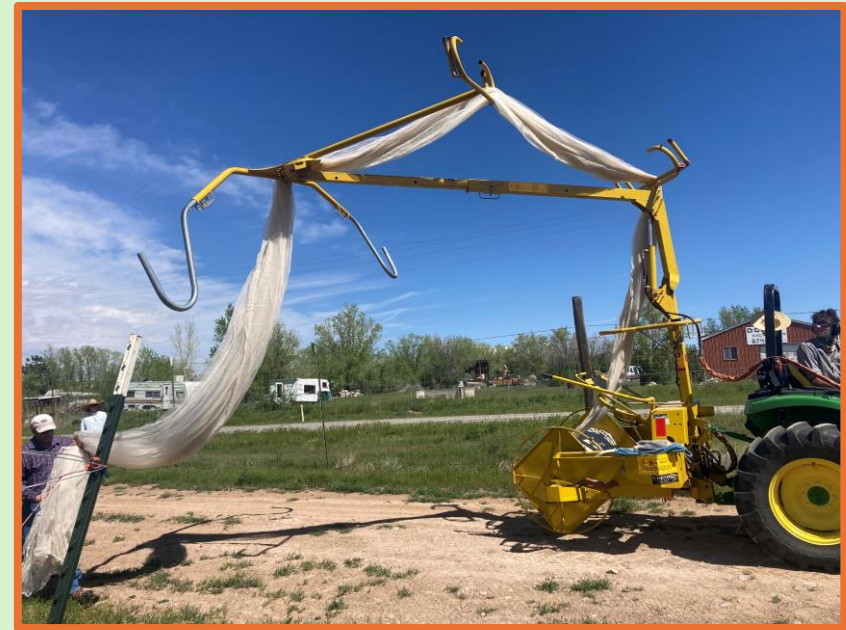
Tractor implement for draping nets over tree rows
